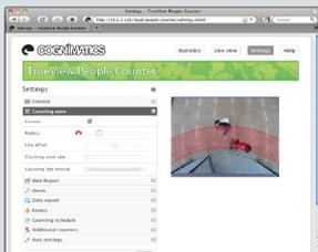
Set all parameters with a minimum of effort and optimize the counting zone using simple slide bars.
